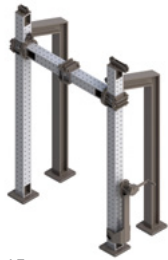
Portal Frame 46.8 kN dynamic max loads (65 kN static) 300-degree Turning Beam width 63 in, extended max height 93 in
