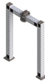
Portal Frame 100 kN dynamic max loads (160 kN static) Standard Beam width 59 in, max height 88 in
