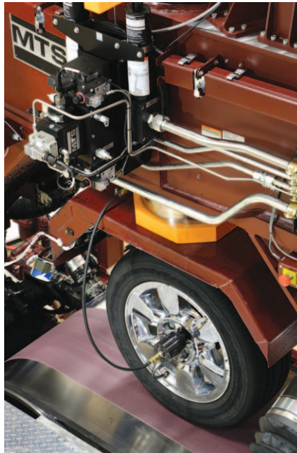
The Flat-Trac LTRe features an electric spindle torque drive that delivers the power density and ultra-high performance bandwidth required to apply driving and braking torque at full roadway speeds, under physical loads up to 30,000 N in all three force directions.
